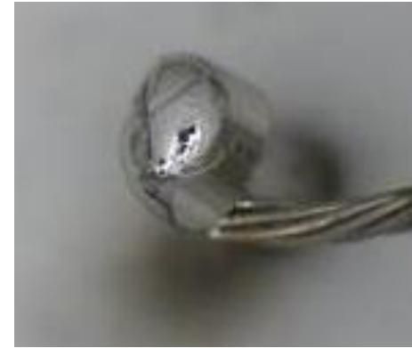
Welded with Pt sleeves
