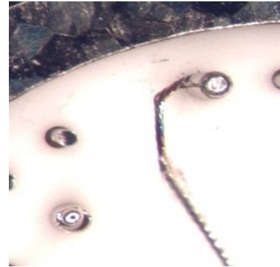
Welded with Pt sleeves
